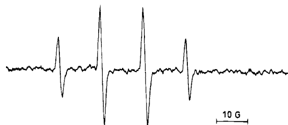
Figure 6. EPR spectrum DMPO/OH radical adducts produced during the thermolysis of MFT-MFT in water.
